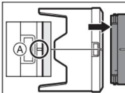
**2 Rotate the lens hood in the direction of the arrow to align mark (B) (○) on the lens hood with the mark on the tip of the lens.**
